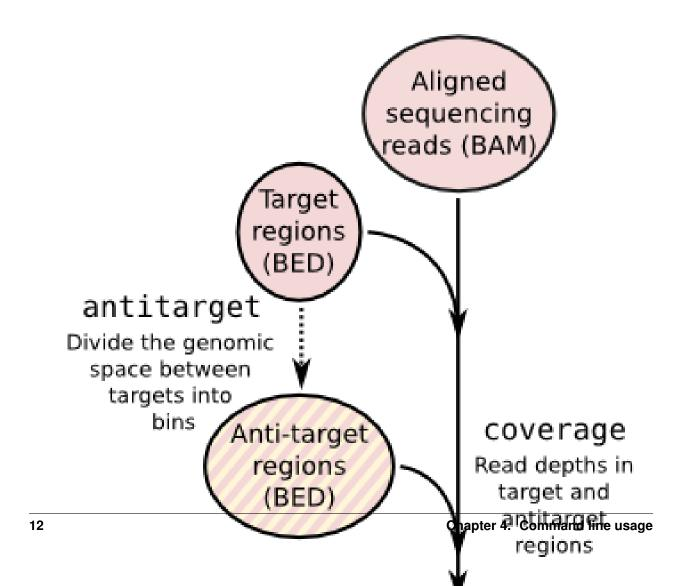
Each operation is invoked as a sub-command of the main script, cnvkit.py. A listing of all sub-commands can be obtained with cnvkit --help or -h, and the usage information for each sub-command can be shown with the --help or -h option after each sub-command name:
